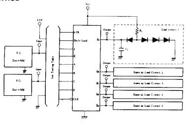
Notes) 1. C<sub>L</sub> includes probe and jig capacitance.
