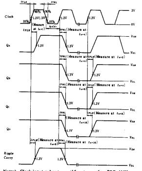
Notes) Ctock input pulse;  $t_{TLH \le 1}$ 15ns,  $t_{THL} \le 6$ ns, PRR = 1MHz, duty cycle=50% and: for  $f_{max}$ ,  $t_{TLH} = t_{THL} \le 2$ .5ns.  $t_n$  is reference bit time when all outputs are low.
