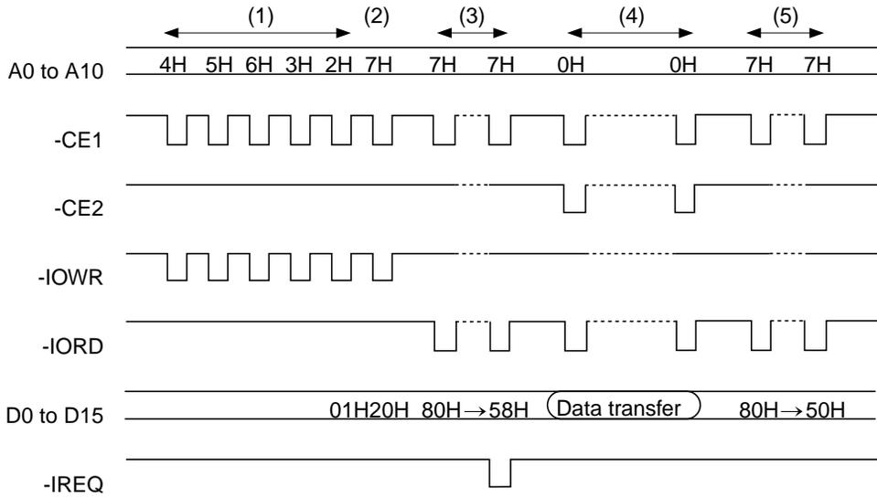
2. Sector write: 1 sector write procedure after the card configured I/O interface is shown as follows.
