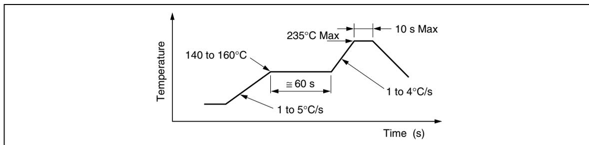
**Figure 1 An Example of Infrared Rays Reflow Conditions**
