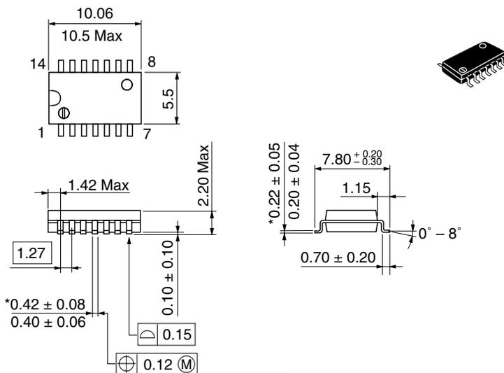
\*Dimension including the plating thickness
