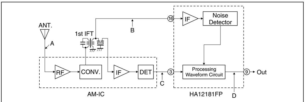
Figure 2 System Block Diagram of AM Radio
