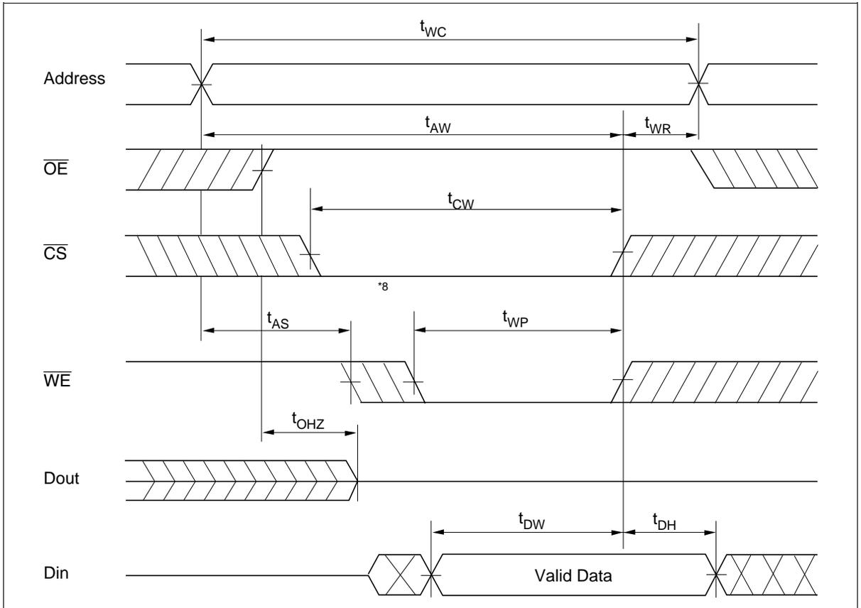
Write Timing Waveform (2) ( $\overline{OE}$  Low Fixed)
