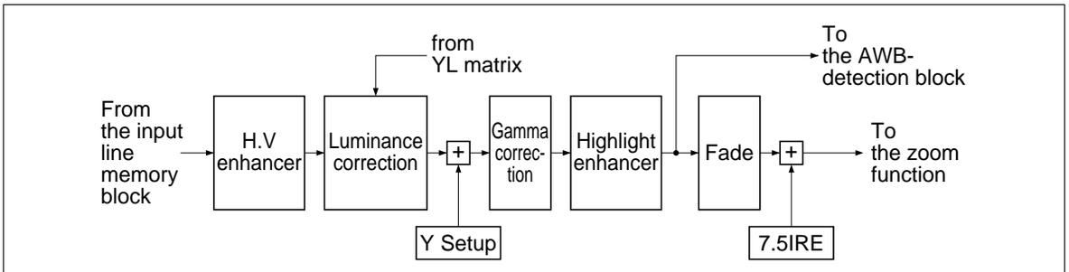
**Figure 5 Luminance-Signal-Processing Block**
