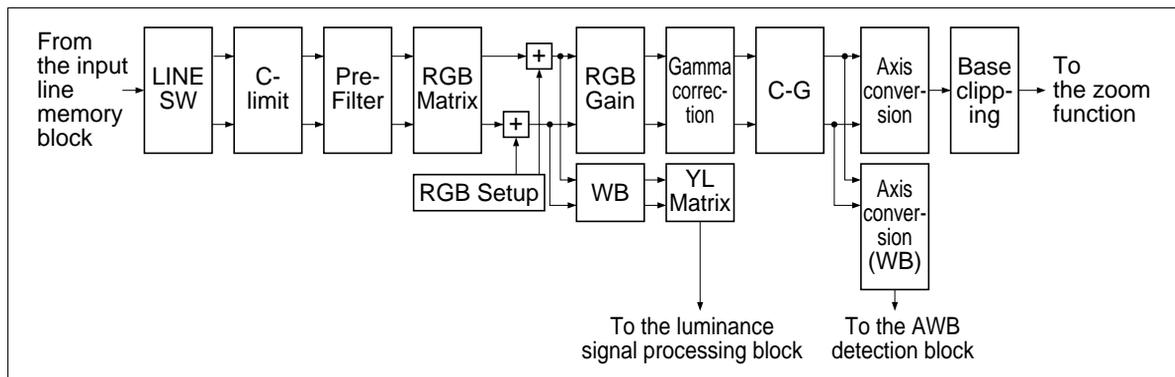
**Figure 4 Color-Signal Processing Block**
