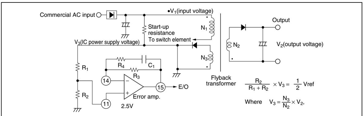
**Figure 1.1 Error Amplifier Peripheral Circuitry Diagram**
