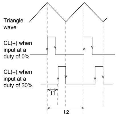
$$Du = \frac{t_1}{t_2} \times 100 (\%)$$
