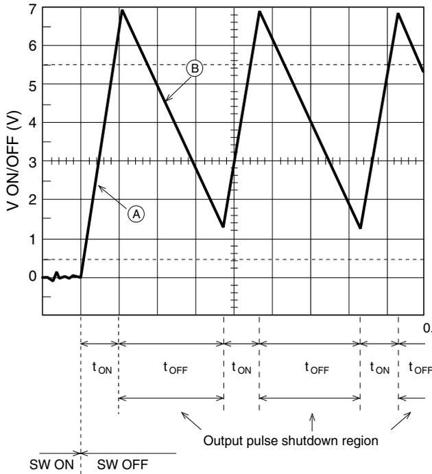
When overcurrent is input at the point where the duty cycle is 30%.
