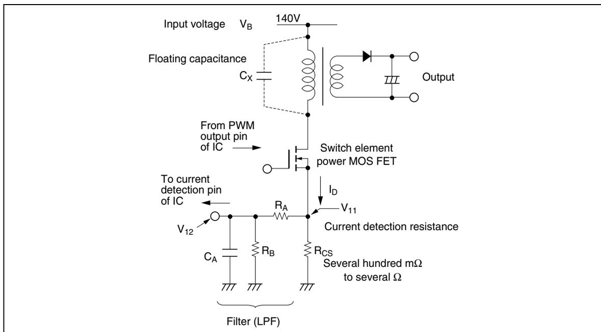
**Figure 2.1 Current Detection Circuit**
