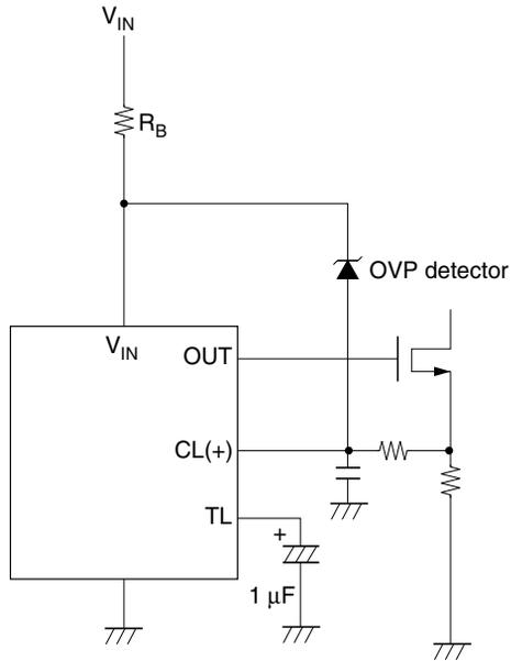
When the OVP detection Zener diode turns on, latch shutdown of the output is performed after the elapse of the time determined by the capacitance connected the TL pin.
