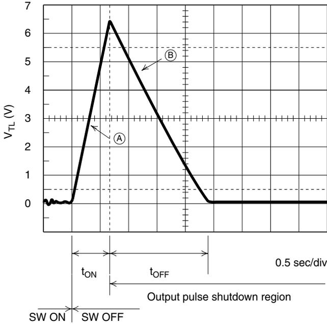
When overcurrent is input at the point where the duty cycle is 30%.
