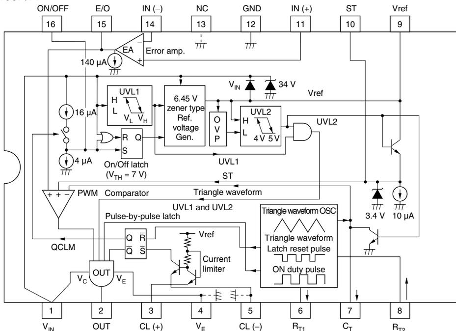
Note: Dotted lines apply to the SOP package model (pins 4, 5, and 13: ground)
