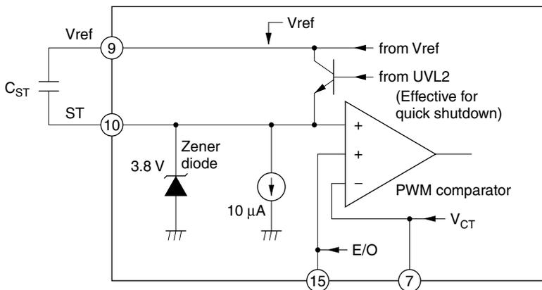
Note: The soft-start time constant is determined by  $C_{ST}$  and the constant-current value (typically 10  $\mu A$ ).
