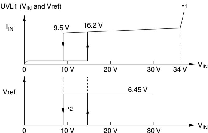
Notes: 1. Breakdown voltage of the internal Zener diode ( $V_Z = 34\text{ V typ.}$ ).
