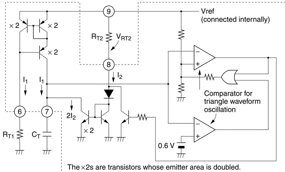
$$I_1 = \frac{V_{ref} - 2V_{BE}}{R_{T1}} \quad t_{DB} = \frac{C_T \times R_{T1} \times 2V}{V_{ref} - 2V_{BE}} \approx 0.4 \times C_T \times R_{T1} \text{ (s)} \quad Du_{max} = \frac{R_{T2}}{2R_{T1}}$$
