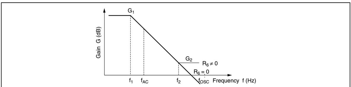
**Figure 1.2 Error Amplifier Characteristic**
