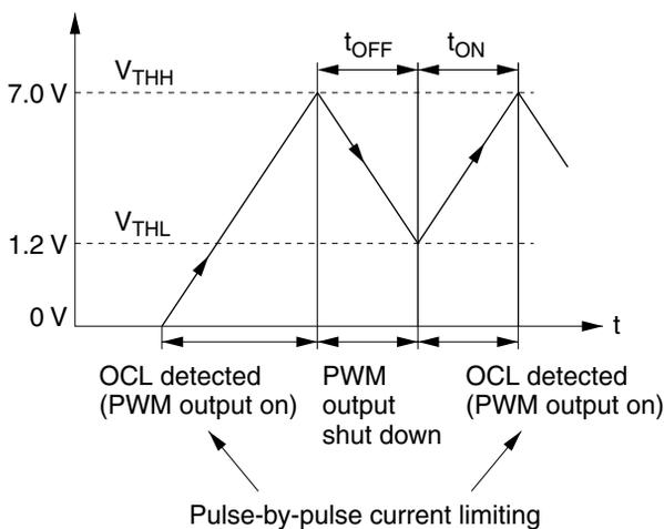
$$t_{ON} \approx \frac{C \times 5.8 V}{(0.9 - Du) \times 16 \mu A - 4 \mu A}$$
