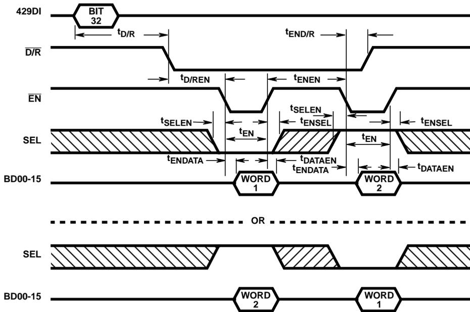
FIGURE 3. RECEIVER TIMING
