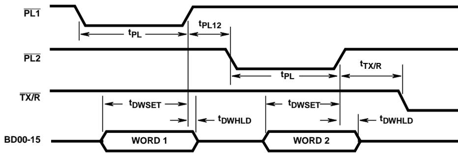
FIGURE 5. TRANSMITTER FIFO WRITE TIMING
