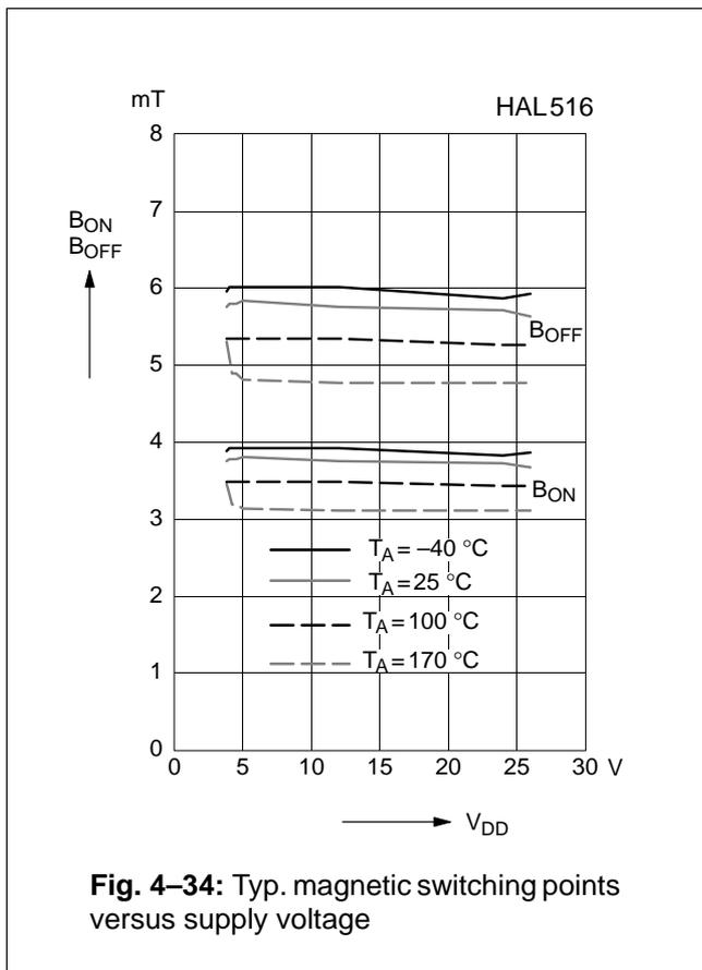
**Fig. 4-34:** Typ. magnetic switching points versus supply voltage
