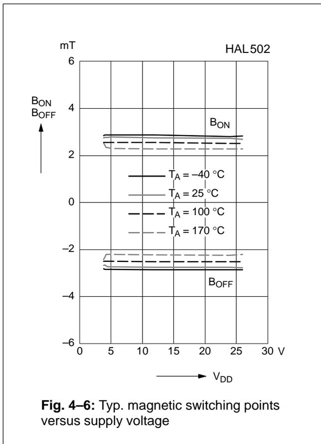
**Fig. 4-6:** Typ. magnetic switching points versus supply voltage
