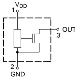
**Fig. 1-1:** Pin configuration
