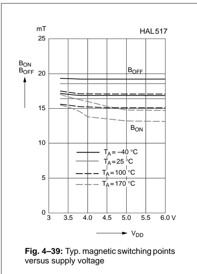
**Note:** In the diagram “Magnetic switching points versus ambient temperature” the curves for  $B_{ONmin}$ ,  $B_{ONmax}$ ,  $B_{OFFmin}$ , and  $B_{OFFmax}$  refer to junction temperature, whereas typical curves refer to ambient temperature.
