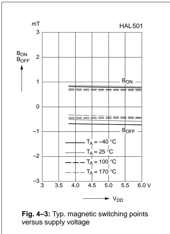
**Fig. 4-3:** Typ. magnetic switching points versus supply voltage
