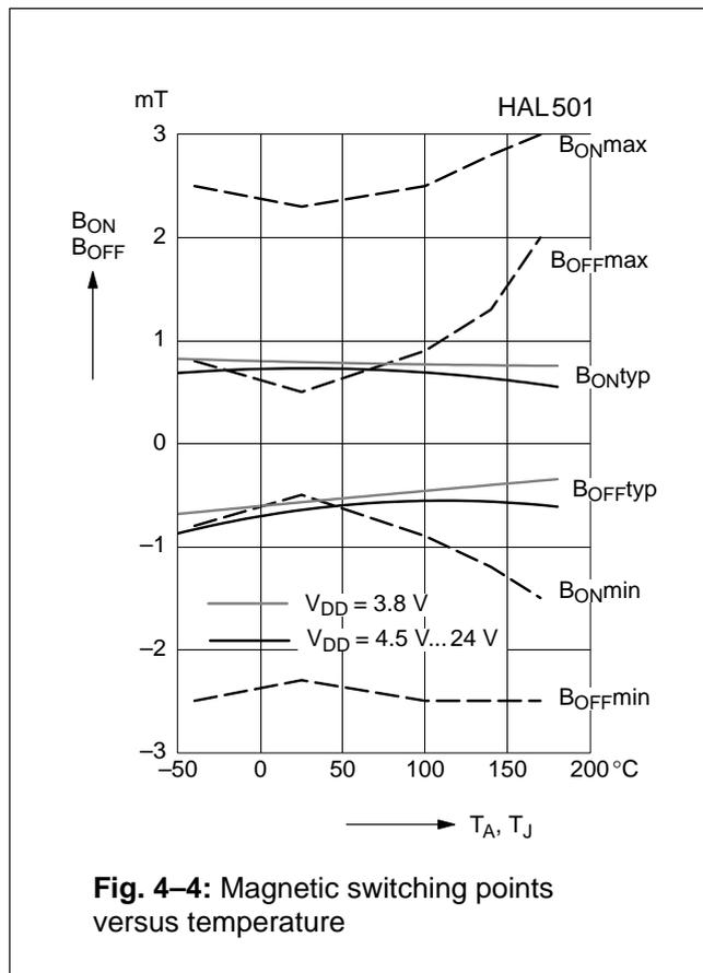
**Fig. 4-4:** Magnetic switching points versus temperature
