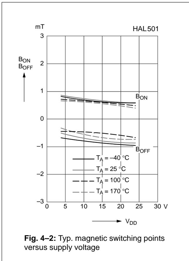
**Fig. 4-2:** Typ. magnetic switching points versus supply voltage
