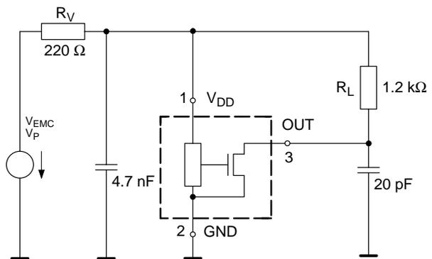
Fig. 5–2: Test circuit 2
