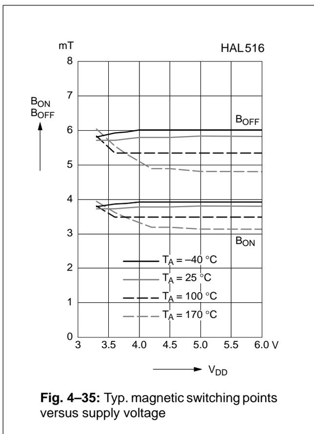
**Fig. 4-35:** Typ. magnetic switching points versus supply voltage
