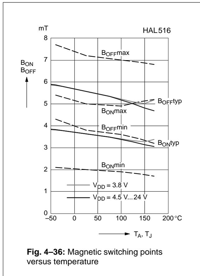
**Fig. 4-36:** Magnetic switching points versus temperature
