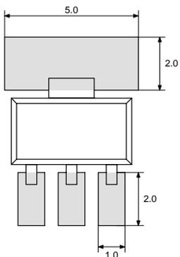
**Fig. 3–4:** Recommended pad size SOT-89x
