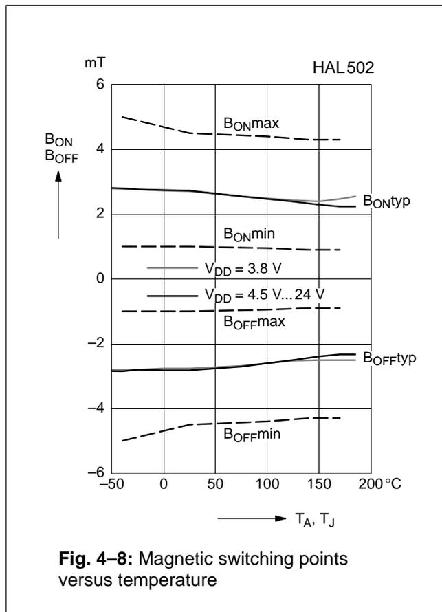
**Fig. 4-8:** Magnetic switching points versus temperature
