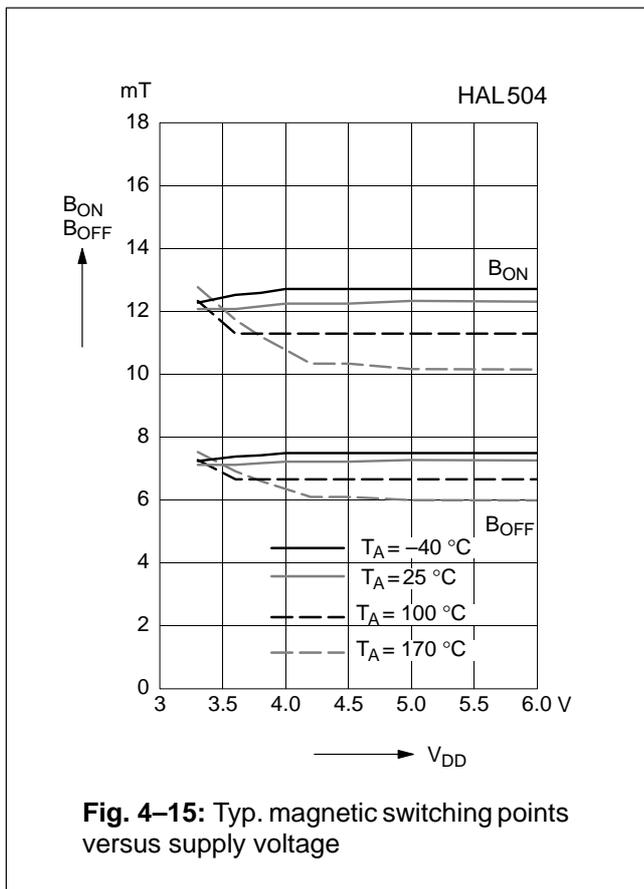
**Fig. 4-15:** Typ. magnetic switching points versus supply voltage
