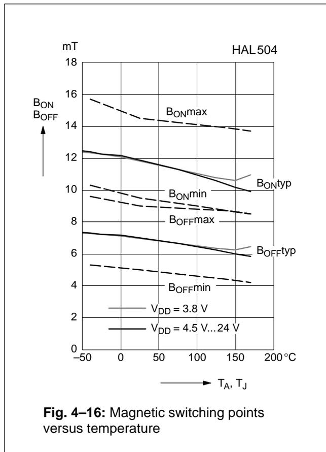
**Fig. 4-16:** Magnetic switching points versus temperature
