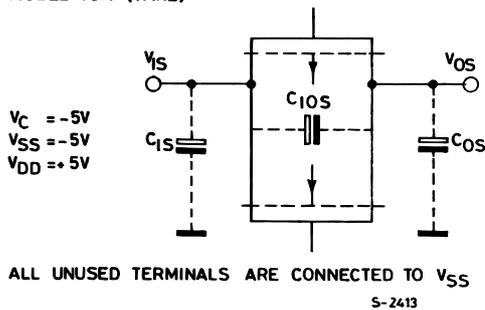
CROSSTALK CONTROL INPUT TO SIGNAL OUTPUT
