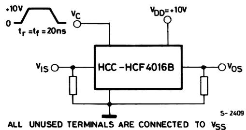
TURN-ON PROPAGATION DELAY-CONTROL INPUT TO OUTPUT
