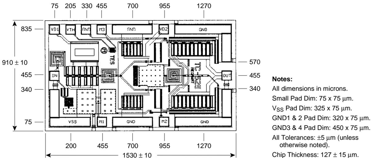
Figure 2. HMMC-5004 Bond Pad Locations.
