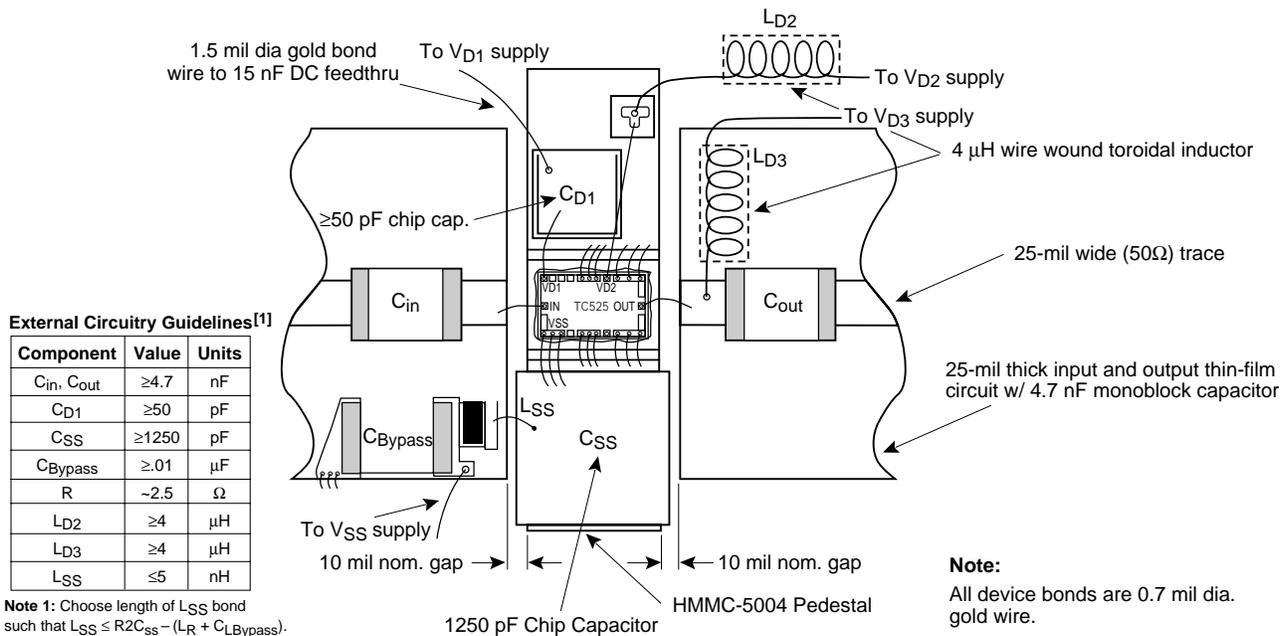
Figure 3. HMMC-5003 Assembly Diagram (for 10 MHz to 3 GHz Operation).
