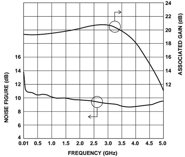
**Figure 7. Typical Noise Figure Performance.**
