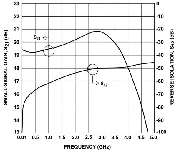
Figure 4. Typical Gain and Reverse Isolation vs. Frequency.
