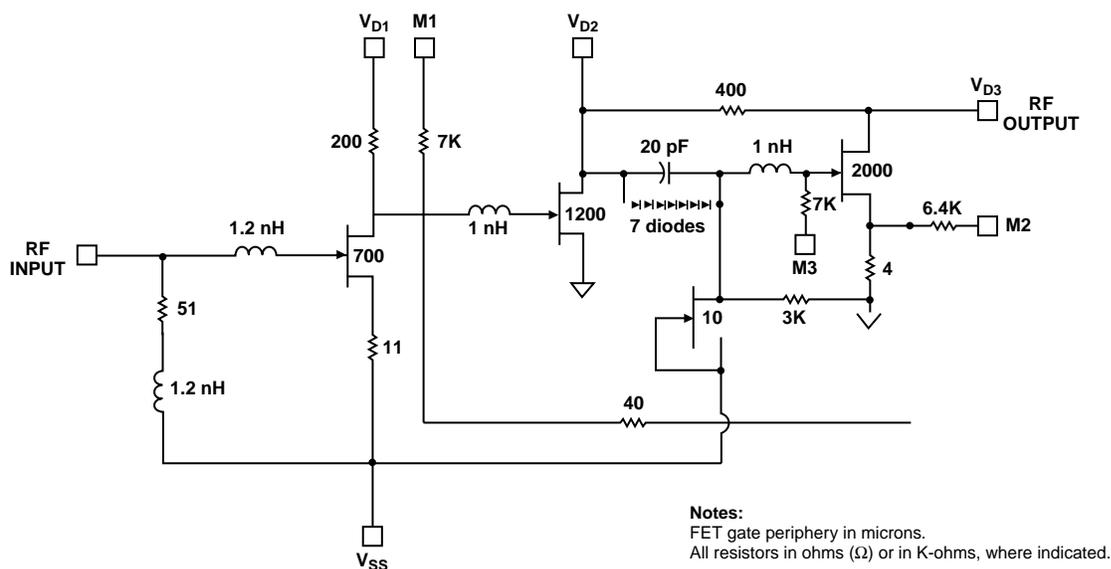
Figure 1. HMMC-5004 Schematic.
