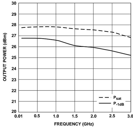
**Figure 8. Typical 1dB Gain Compression and Saturated Output Power vs. Frequency.**
