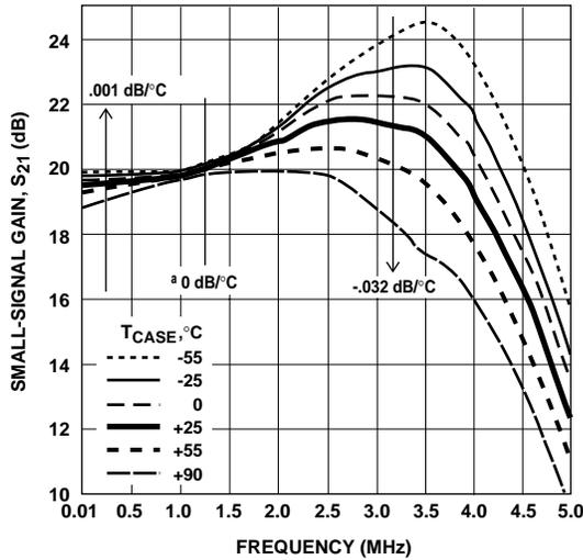
**Figure 6. Typical Small-Signal Gain vs. Temperature.**
