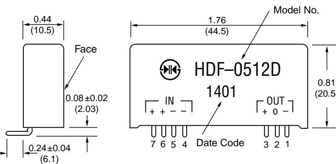
With optional formed leads available - use "F suffix." Dimensions in inches; ( ) Dimensions in mm.
