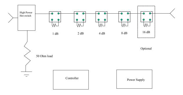
Figure 1 High Power Step Attenuator
