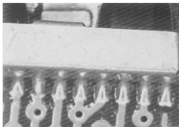
Photo 4.0. Unit self-aligns after reflow.
