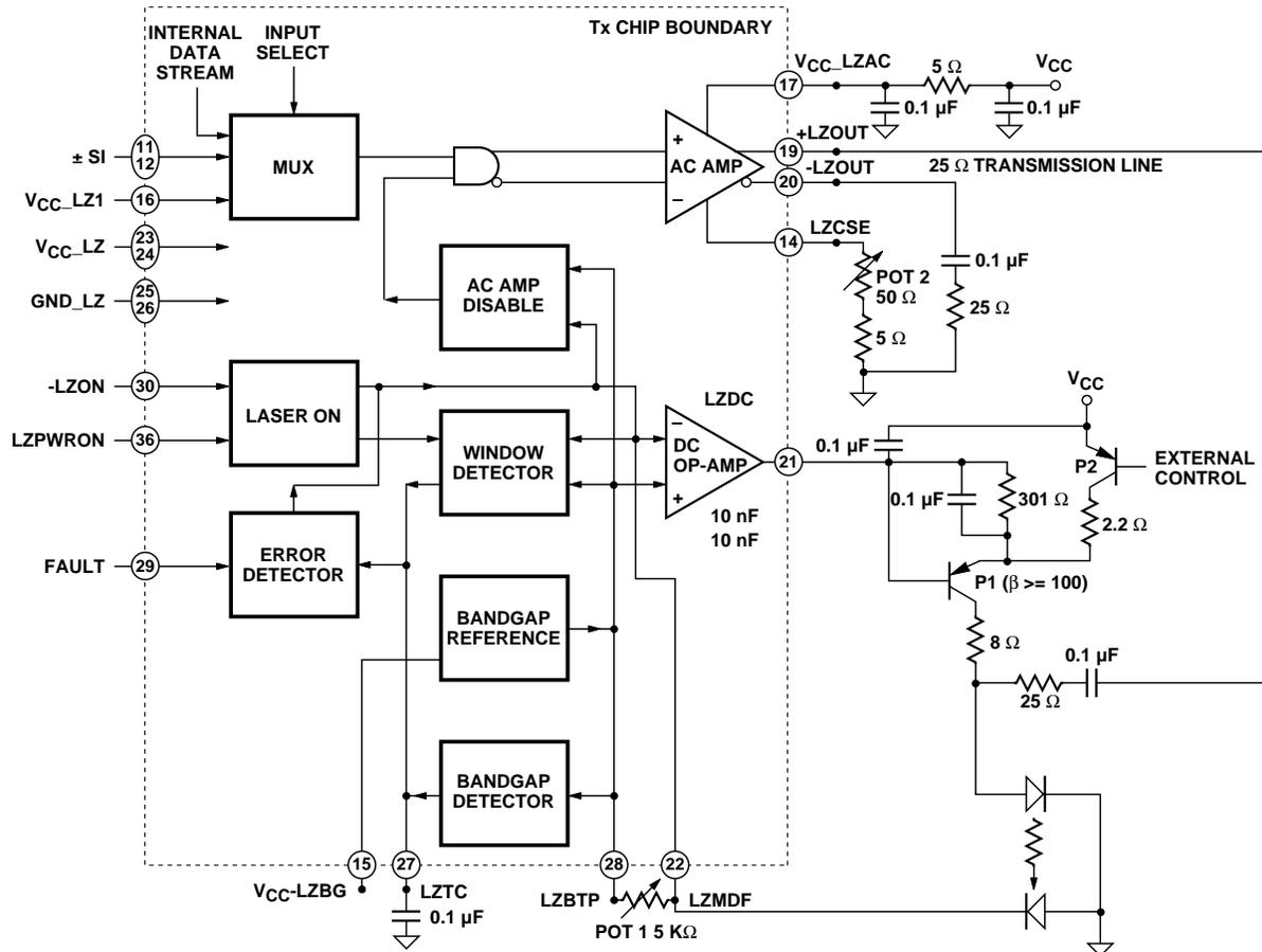
Figure 3. Laser Driver Block Diagram and External Circuitry.
