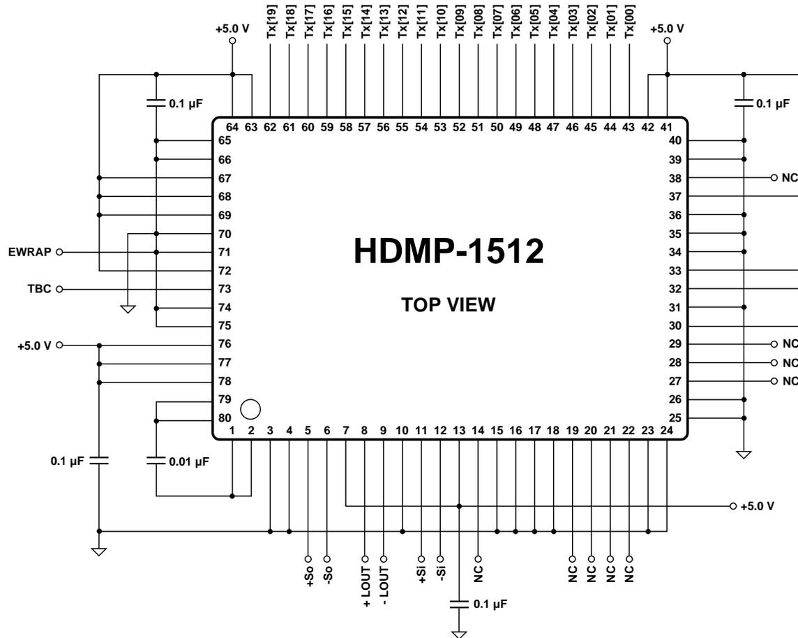
**Figure 18. Typical Transmitter Pin Terminations for Applications Requiring High Speed Serial Copper Drivers ( $\pm$  So). Laser Driver Outputs Are Disabled. For 1062.5 MBd Operation Only, SPDSEL (pin 67) Set High, Non Ping-Pong Mode (PPSEL = 0).**
