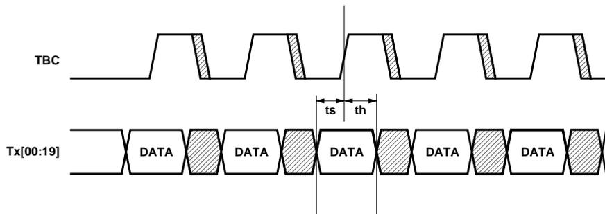
Figure 14. HDMP-1512 (Transmitter) Timing Diagram, with PPSEL = 0.
