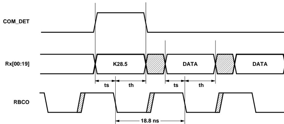
Figure 15. HDMP-1514 (Receiver) Timing Diagram, with PPSEL = 0.
