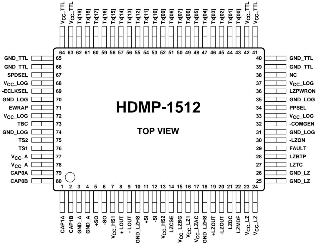
Figure 11. HDMP-1512 (Tx) Package Layout, Top View.
