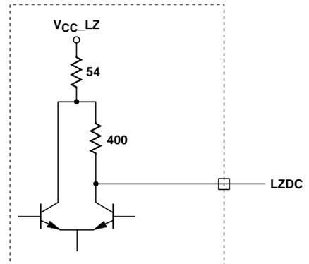
Figure 4. LZDC Equivalent Output Circuit (Tx pin # 21).
