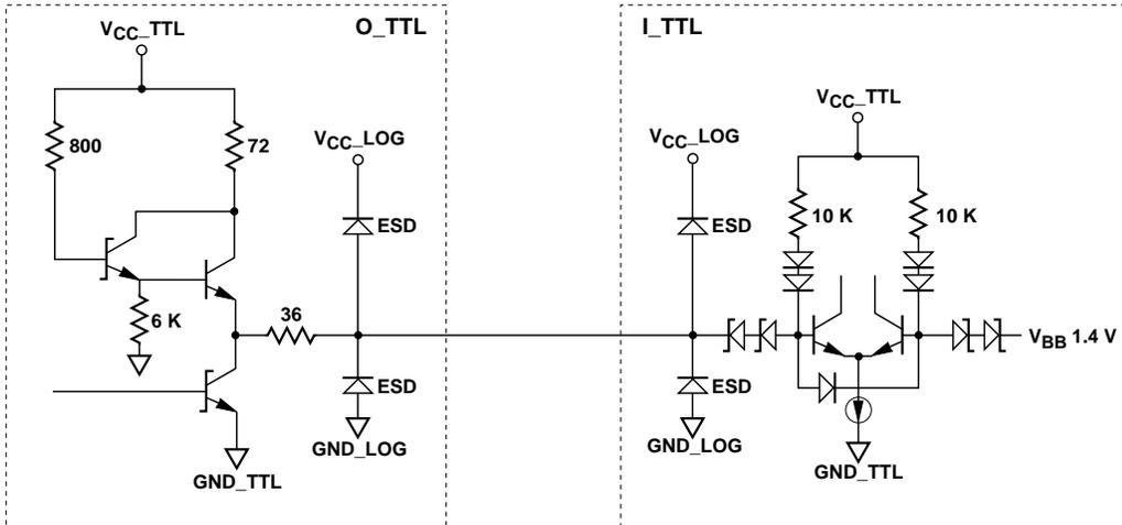
Figure 9. O-TTL and I-TTL Simplified Circuit Schematic.
