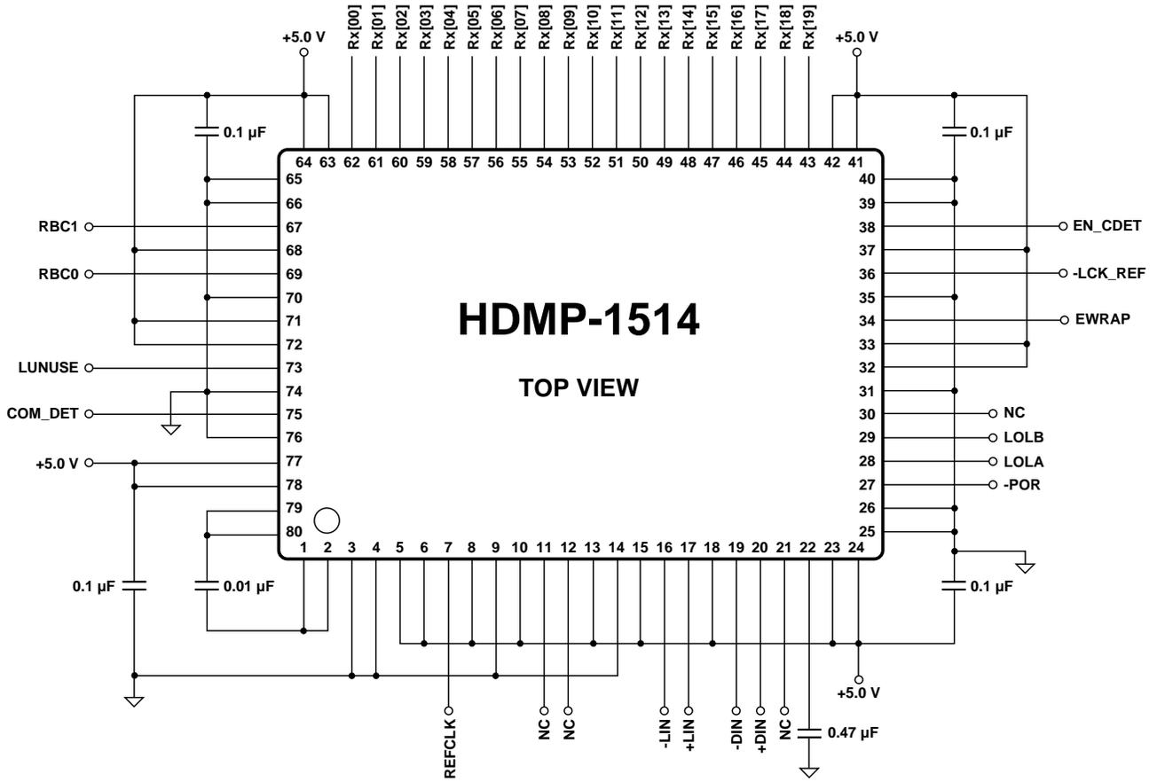
**Figure 20. Typical Receiver Pin Terminations for Applications Using High Speed Serial Copper Links ( $\pm$  DIN). For 1062.5 MBd Operation Only, SPDSEL (pin 71) Set High, Non Ping-Pong Mode (PPSEL = 0).**
