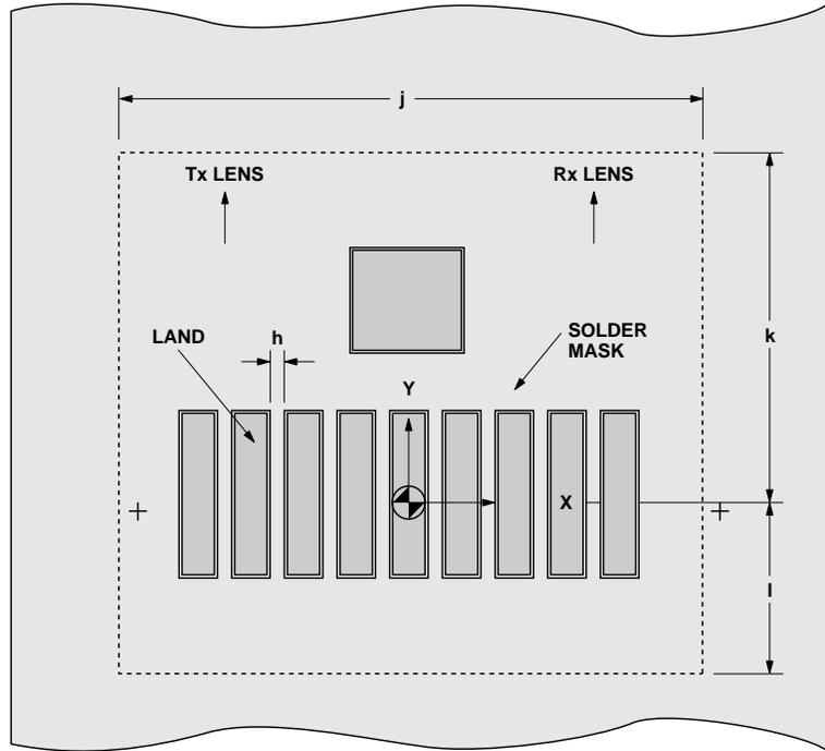
Figure 3. PCBA – Adjacent land keep-out and solder mask.
