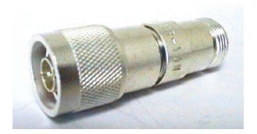
The Microlab/FXR HR series of DC Blocks is used to prevent the flow of direct current and low frequency current surges along the inner and/or the outer conductors of a transmission line, while permitting the unimpeded flow of RF signals. Applications include the blocking of current surges that can occur in subway tunnels and at antenna sites during lightening storms or whenever DC isolation is required.
