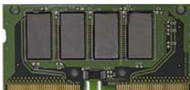
Figure 1: HCD SO-RIMM™ Module without Heat Spreader (Note: 4 additional RDRAMs are installed on the back side of the PCB)
