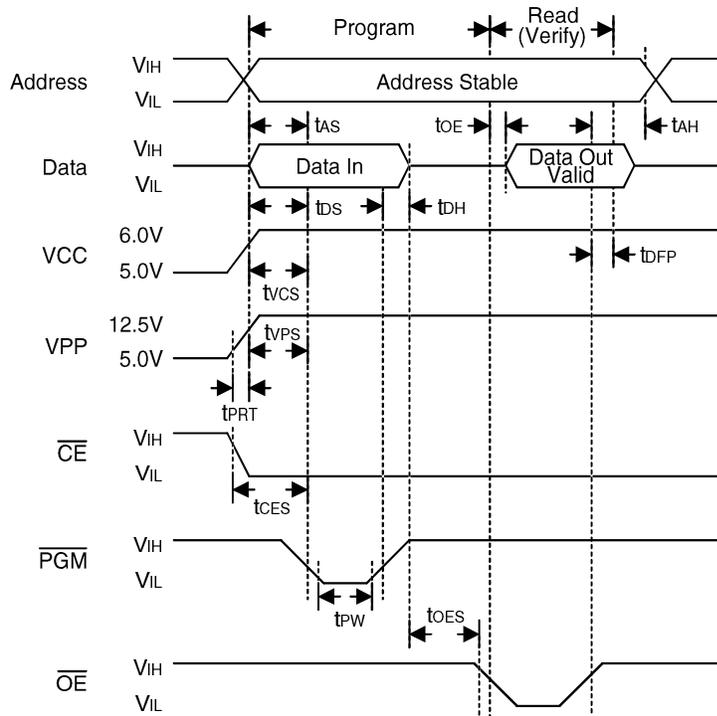
Figure 2. Programming waveforms
