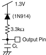
Note: C<sub>L</sub>=100pF including jig capacitance, except for the -45 devices, where C<sub>L</sub>=30pF.
