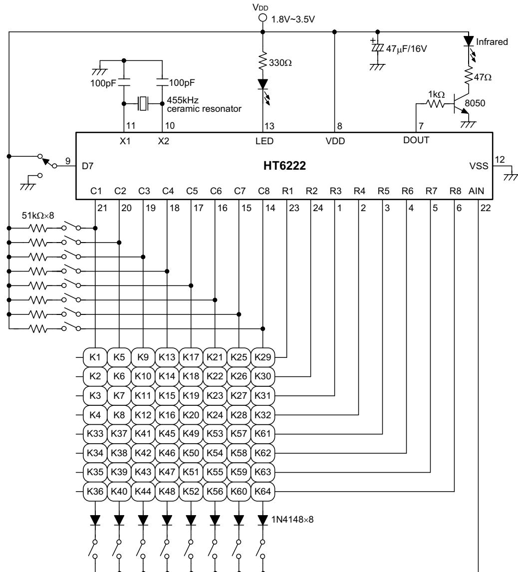
Note: Typical infrared diode: EL-1L2 (KODENSHI CORP.)
