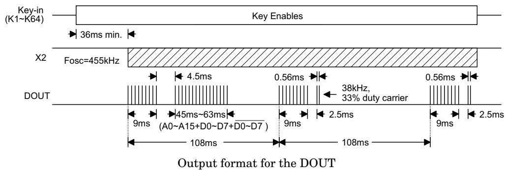
The output code carrier of the DOUT pin is shown in Timing 2:
