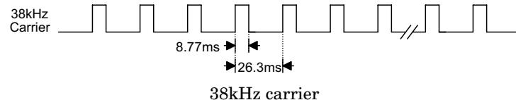
The transmission codes employ the PPM (Pulse Position Modulation) method to represent their two logic states by "0" (1.12ms) and "1" (2.24ms) as shown in Timing 3:
