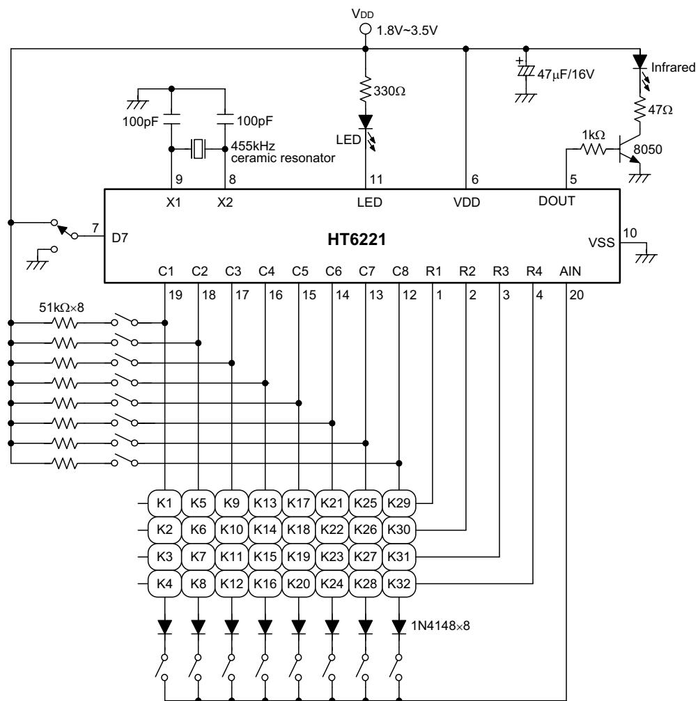
Note: Typical infrared diode: EL-1L2 (KODENSHI CORP.)
