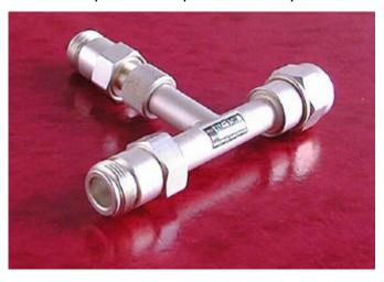
Microlab/FXR HZ-15 series is a reactive tap/sampler designed for either tapping off 10 dB or less power to a side track in a radiating cable system or for sampling/monitoring wireless carriers between base station radio and antenna.
