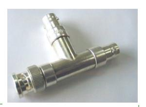
Microlab/FXR Model HM series resistive samplers consist of a resistive attenuator coupled to a short length of  $50\Omega$  transmission line. A small portion of the RF energy in the main line is coupled through the attenuator to the auxiliary output, the balance being transmitted to the output with negligible reflection or loss. The coupling is fixed, non-directional and independent of frequency over an extremely broad bandwidth.
