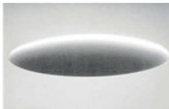
Micro-Machined Lens in InP Die Surface
