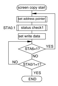
This command is available when hardware column number and software column number are the same. Hardware column number is related to MD2 and MD3 setting. Software column number is related to set text area and set graphic area command.
