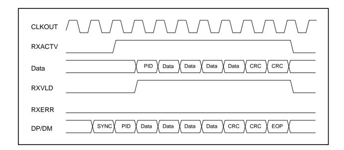
Note that the USB 2.0 transceiver does not decode Packet ID's (PIDs). They are passed to the SIE for decoding.
