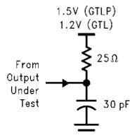
$C_L$  includes probes and jig capacitance.
