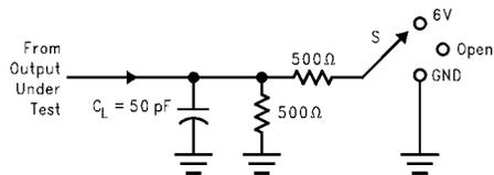
$C_L$  includes probes and jig capacitance.
