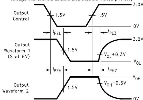
Waveform 1 is for an output with internal conditions such that the output is low except when disabled by the output control. Waveform 2 is for an output with internal conditions such that the output is high except when disabled by the output control. All input pulses have the following characteristics: frequency = 10 MHz,  $t_r = t_f = 2$  ns,  $Z_0 = 50\Omega$ . The outputs are measured one at a time with one transition per measurement.
