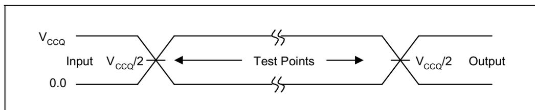
NOTE: AC test inputs are driven at  $V_{CCQ}$  for a Logic "1" and 0.0 V for a Logic "0." Input timing begins, and output timing ends, at  $V_{CCQ}/2$  V (50% of  $V_{CCQ}$ ). Input rise and fall times (10% to 90%) < 5 ns.
