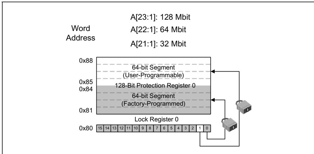
**NOTE:** A0 is not used in x16 mode when accessing the protection register map (See Table 8 for x16 addressing). For x8 mode A0 is used (See Table 9 for x8 addressing).
