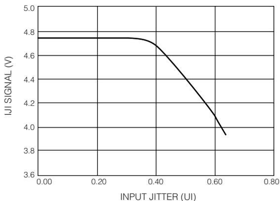
Fig. 21 Input Jitter Indicator (Typical at  $T_A = 25^\circ\text{C}$ )
