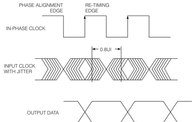
Fig. 16 Phase Detector Characteristics
