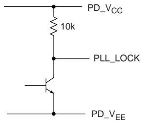
All on-chip resistors have  $\pm 20\%$  tolerance at room temperature.
