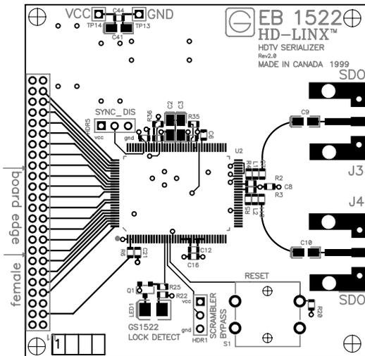
Fig. 28 Top Layer of EB1522 PCB Layout
