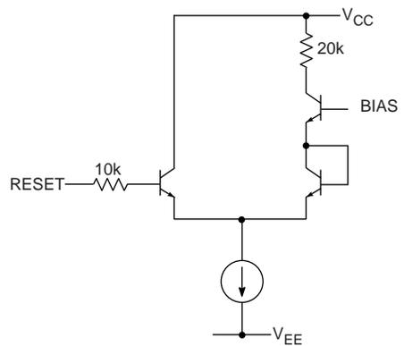
Fig. 12 RESET Circuit
