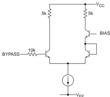
Fig. 13 BYPASS Circuit
