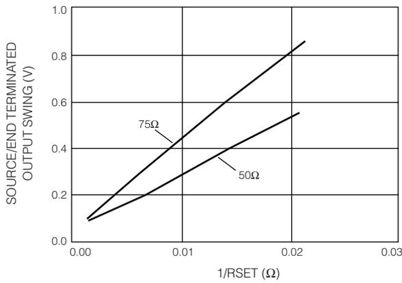
Fig. 23 Signal Swing for Various  $R_{SET}$  Admittances
