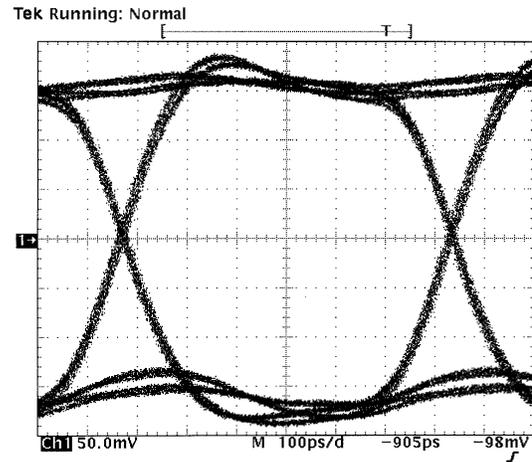
Fig. 24 Uncompensated Output Eye Waveform
