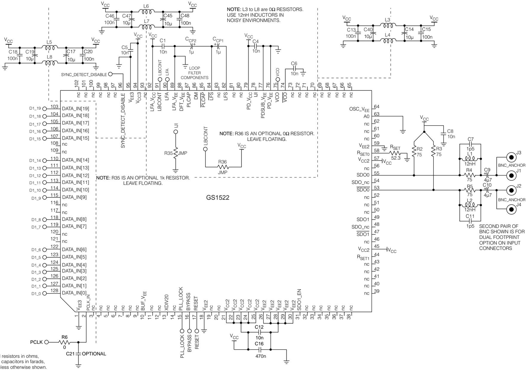
All resistors in ohms, all capacitors in farads, unless otherwise shown.
