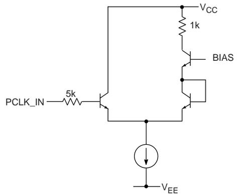
Fig. 11 PCLK\_IN Circuit
