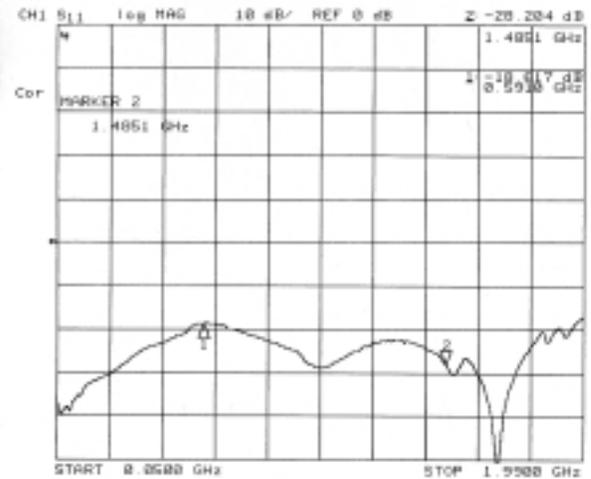
Fig. 26 Compensated Output Return Loss at Logic HIGH
