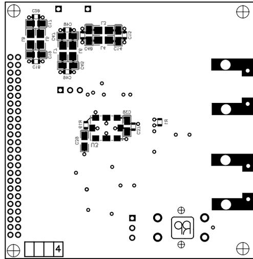
Fig. 31 Bottom Layer of EB1522 PCB Layout
