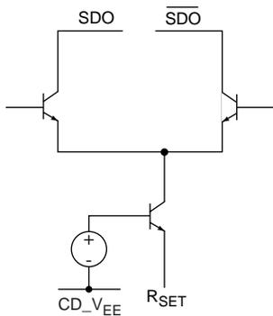
Fig. 9 SDO/SDO Output Circuit
