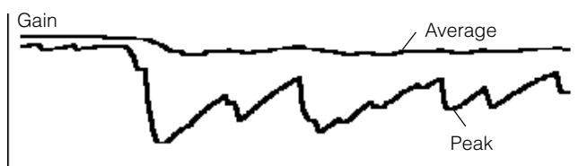
Fig. 7 Gain versus Time - Average and Peak Detectors
