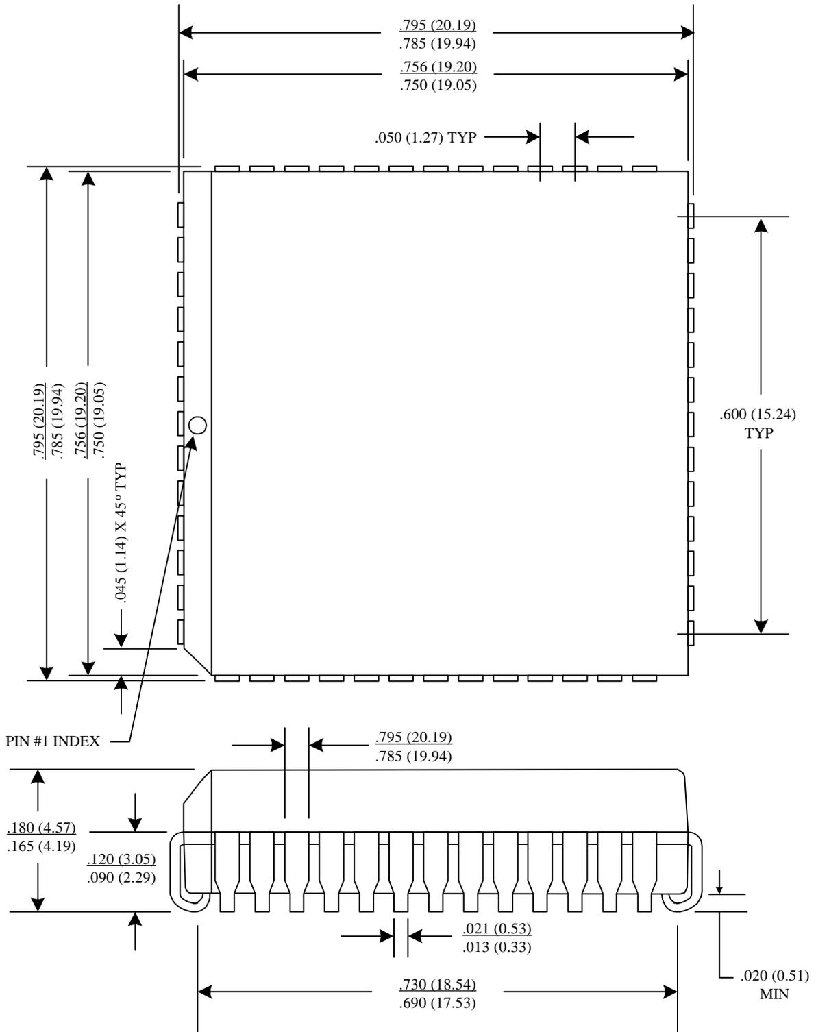
Note: All dimensions in inches (millimeters)  $\frac{\text{MAX}}{\text{MIN}}$  or typical where noted.
