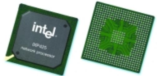
With their Development Platform, a choice of operating systems, and a broad range of development tools, the Intel IXP425 network processors provide a complete development environment for faster time-to-market. This network processor family offers the choice of multiple clock speeds at 266, 400, and 533 MHz, with both Commercial (0° to 70° C) and Extended (-40° to 85° C) temperature options.
