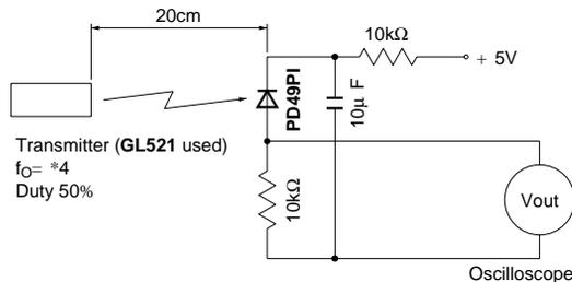
In the above figure, the transmitter should be set so that the output V<sub>out</sub> can be 40mV<sub>p-p</sub>.
