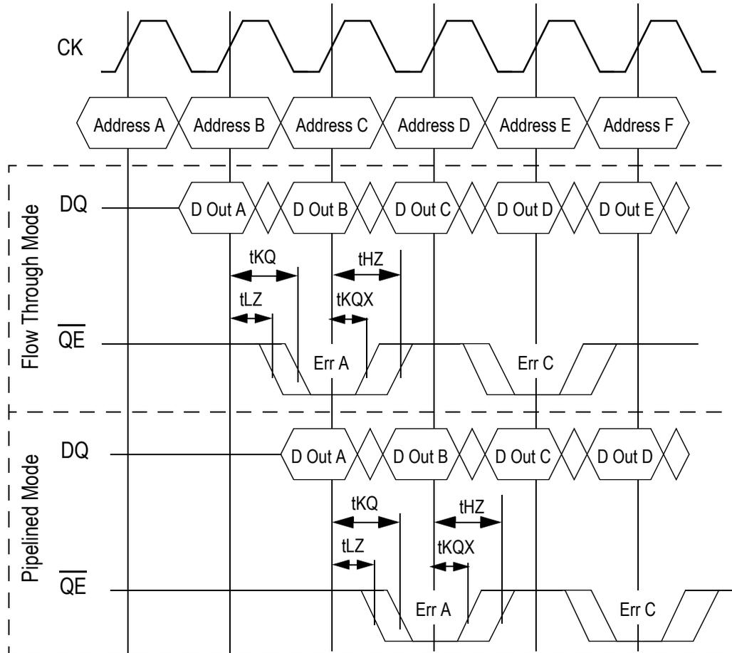
**x18/x36 Mode (PE = 0) Write Parity Error Output Timing Diagram**
