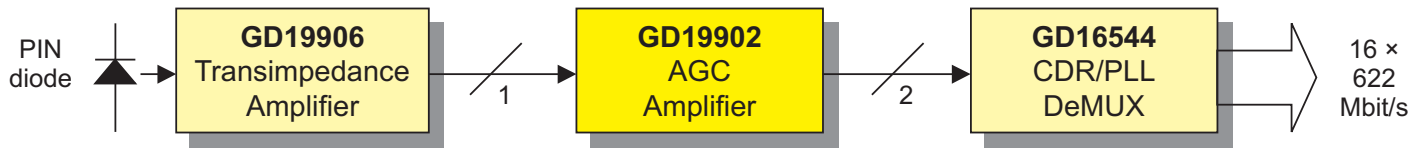
Figure 4. Building blocks for a 10 Gbit/s reception system.
