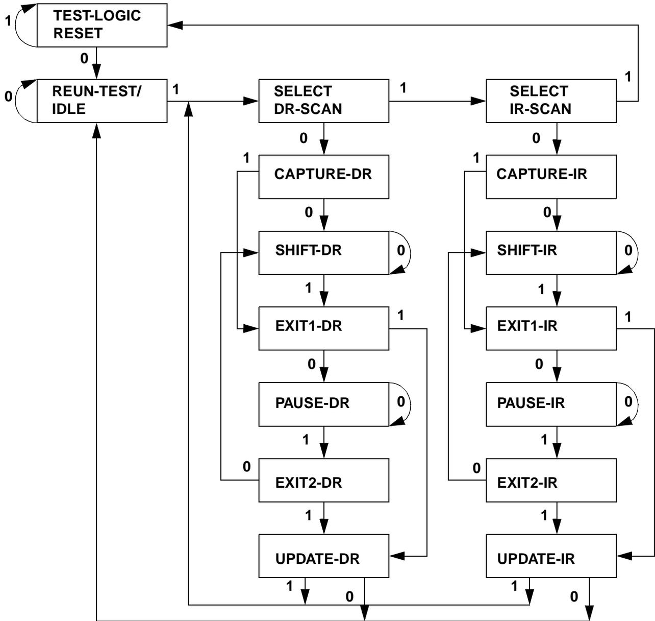
Figure 1. TAP Controller State Diagram<sup>[10]</sup>
