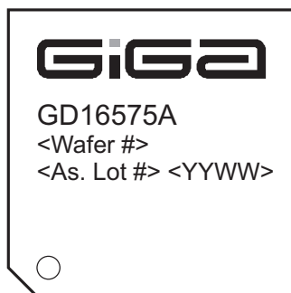
Figure 5. Device Marking, 32 pin Package - Top View
