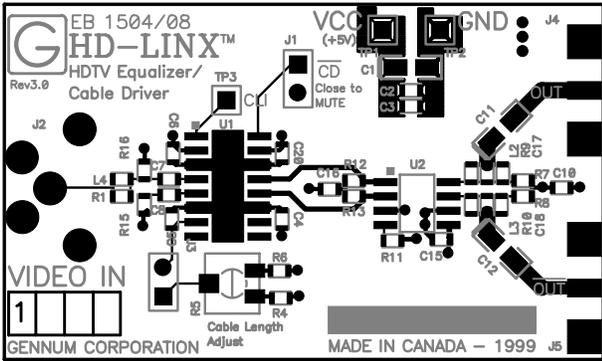
Fig. 30 Top Layer of EB1504/08 PCB Layout
