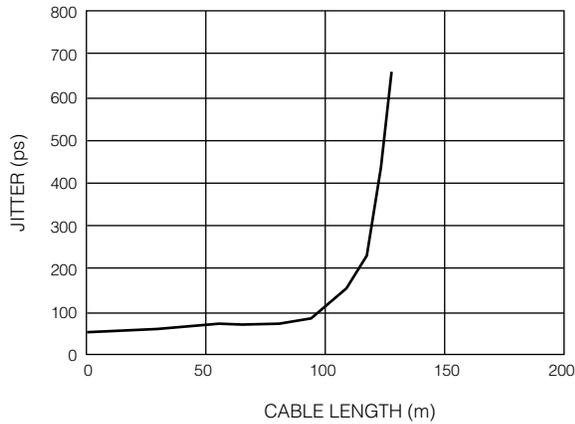
Fig. 9 Typical Peak to Peak Jitter, PRN 2<sup>23</sup>-1, Belden 8281
