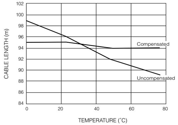
Fig. 11 Typical 1694A Cable Length vs. Temperature
