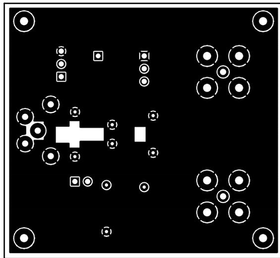
Fig. 25 Ground Layer of EB1504 PCB Layout
