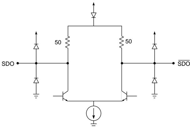
Fig. 4 Output Circuit
