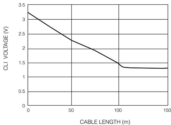
Fig. 20 CLI Voltage vs. Belden 8281 Cable Length
