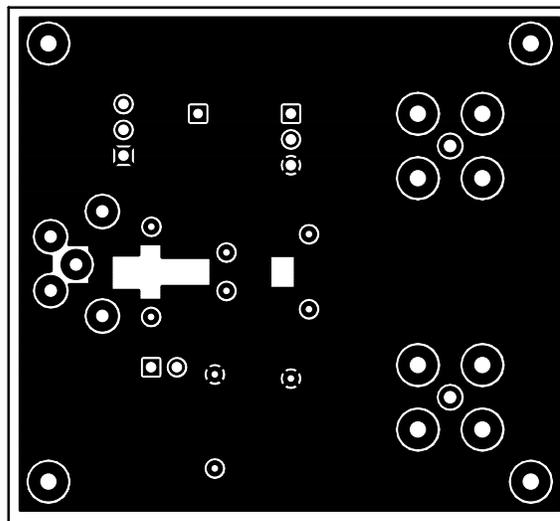
Fig. 27 Power Layer of EB1504 PCB Layout
