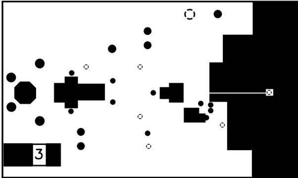
Fig. 31 Power Layer of EB1504/08 PCB Layout
