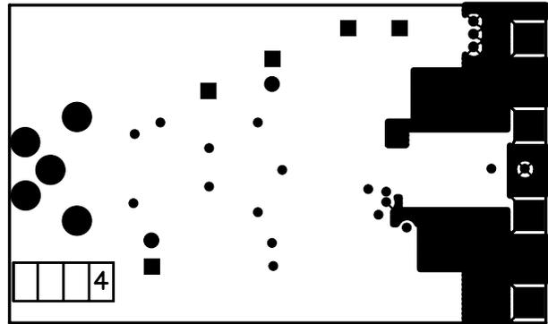
Fig. 33 Bottom Layer of EB1504/08 PCB Layout
