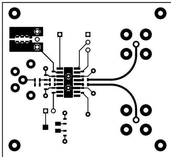
Fig. 24 Top Layer of EB1504 PCB Layout
