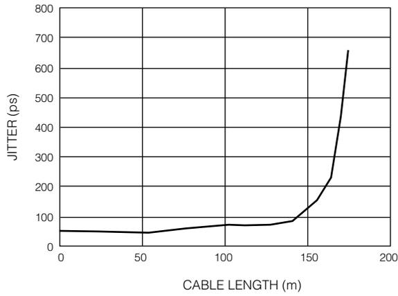
Fig. 8 Typical Peak to Peak Jitter, PRN 2<sup>23</sup>-1, Belden 1694A
