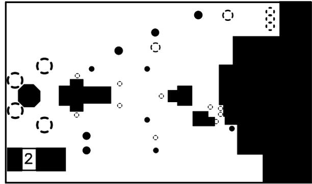
Fig. 32 Ground Layer of EB1504/08 PCB Layout
