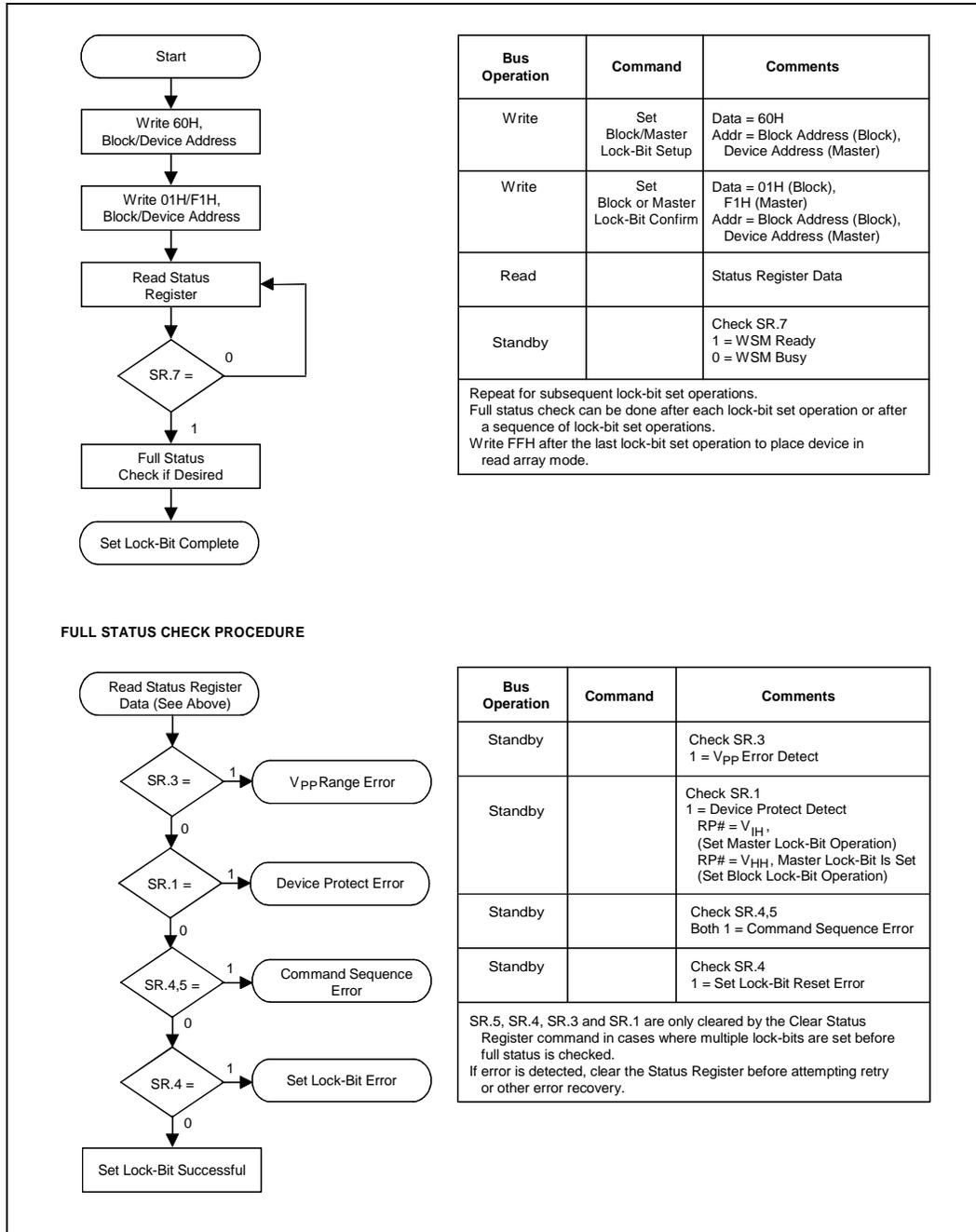
Figure 11. Set Block and Master Lock-Bit Flowchart
