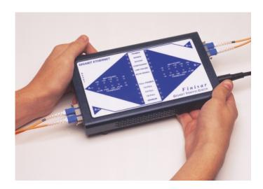
Connect the GT-C to either copper or optical links by using industry-standard Gigabit Interface Converter modules (GBICs). You can change the media type in seconds. Media may be mixed, effectively creating a media converter, changing from a copper interface in one end to an optical interface in the other, for example. The GT-C can also extend links to 10 km by using single-mode, long-wavelength GBICs between two units.
