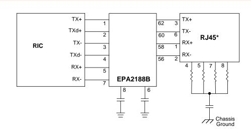
Notes: \* Pin-outs shown are for multiport, DCE configurations: e.g. Hubs, Repeaters
