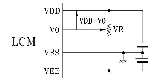
\*VDD-V0: LCD 驱动电压      VR: 10K ~20K
