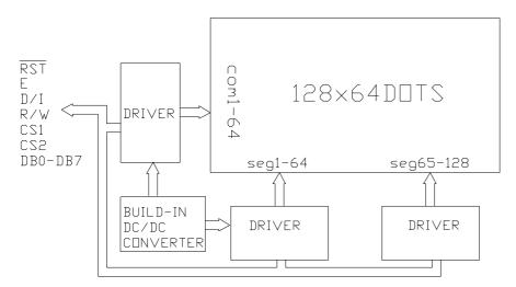
Note: It is necessary to guard all signals from external noise as signal lines are directly connected to C-MOS and are not pull-up or pull-down internally.
