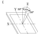
Inspection should be performed within  $\emptyset$  ( $\emptyset$ =30°) from Z axis to each X and Y axis.
