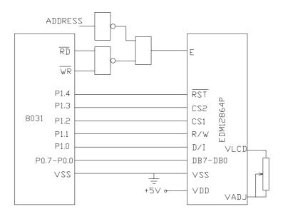
The data bus P0 of 8031 is directly connected to the data bus of module. RD and WR of 8031 act as read/write control signal, interfaced to E signal terminal of module by NAND gate.
