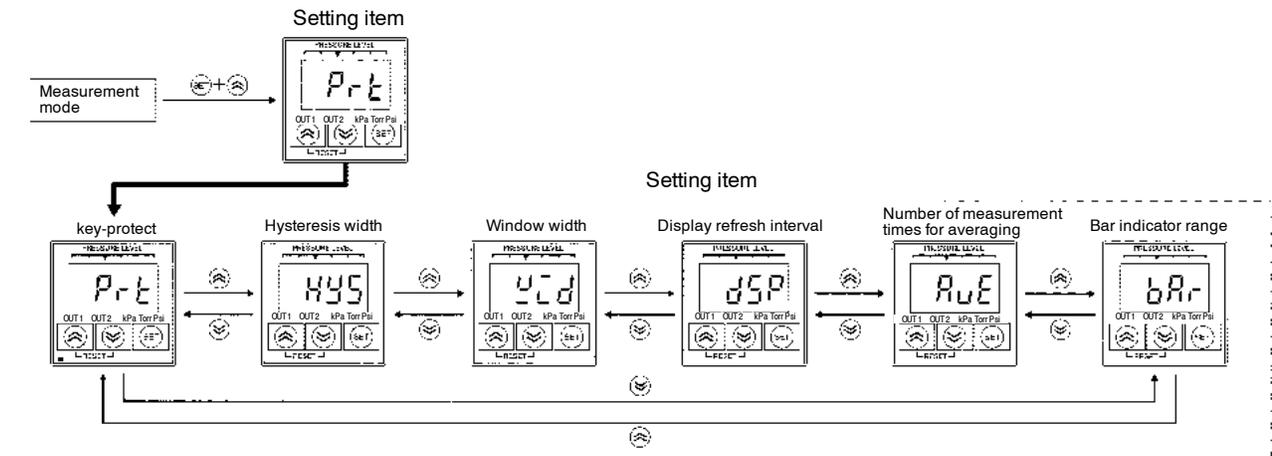
1. Press the SET key and Up key simultaneously to set the E8F2 to special setting mode and display *PrL*.
