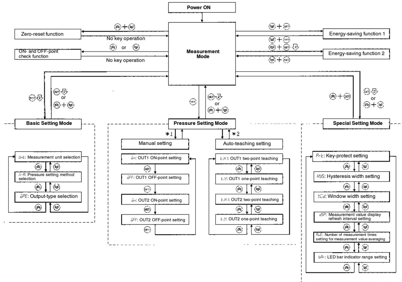
**Note: 1.** and indicate that the key must be pressed for approximately 2 or 3 s respectively.
