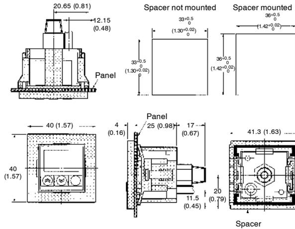
**Note:** The spacer can be removed from the panel-mounting bracket. The panel cutout dimensions can be adjusted as shown above by attaching or detaching the spacer.
