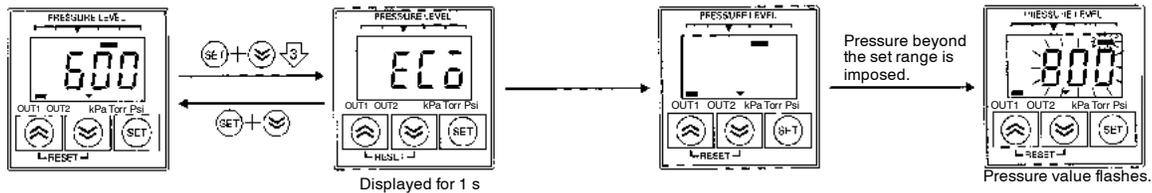
1. If the SET and Down keys are pressed simultaneously for approximately 3 s in measurement mode, ECo will be displayed for 1 s and then the numeric and menu display will be turned OFF.
