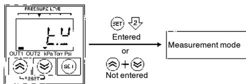
1. Press the SET key under condition 3 below while *E.U.* is displayed to display the present measurement value.
