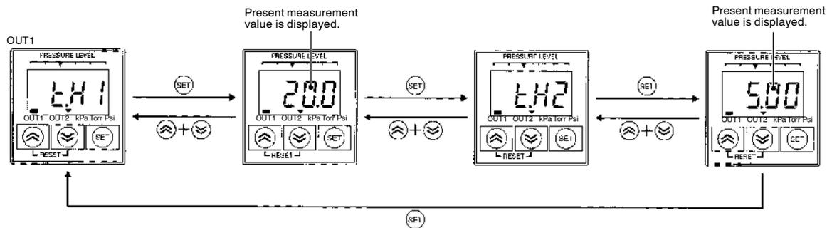
1. Press the SET key under condition 1 below while *L.H.I.* is displayed to display the present measurement value.
