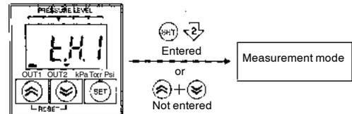
4. Check the measurement value and press the Set key to perform and complete teaching the second point.
