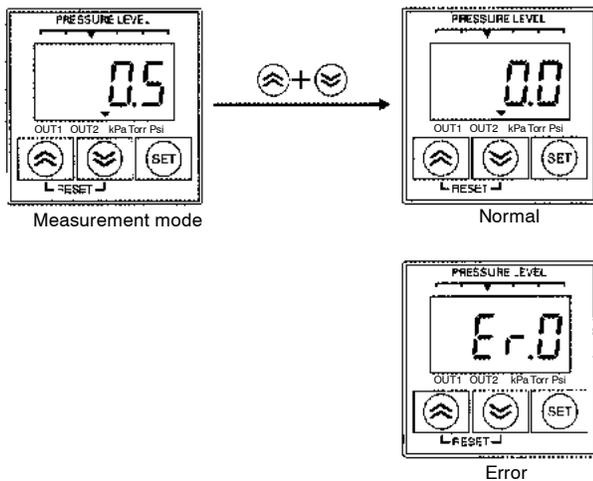
The displayed measurement value is reset to 0 by pressing the Up and Down keys simultaneously. The reset range is within  $\pm 5\%$  (FS) of the rated pressure. If the value is not within the range, an error will be displayed and the reset will not be enabled.
