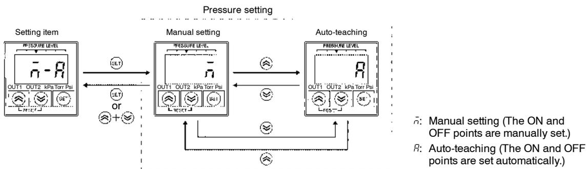
1. Press the SET key while  $\bar{n}-\bar{A}$  is displayed to display the pressure setting method presently set.
