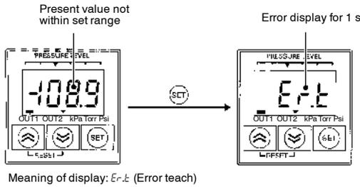
If the present value or the result of calculation after teaching is not within the range, the SET key input will not be accepted. In this case an error will be displayed for 1 s if teaching is performed.
