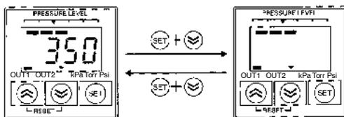
1. The numeric and menu display is turned OFF by pressing the SET and Down keys simultaneously in measurement mode.
