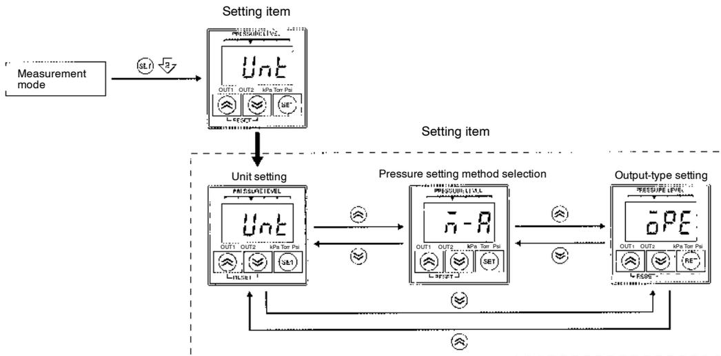
1. Press the SET key for approximately 2 s so that the E8F2 will be set to basic setting mode and *Unt* will be displayed.
