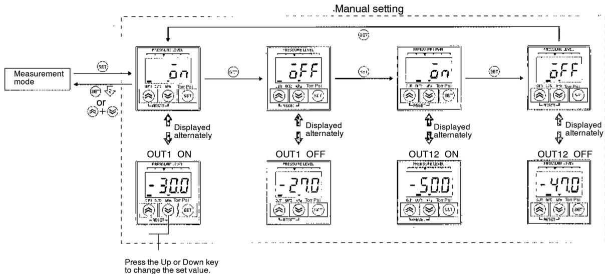
1. Press the SET key, to set the E8F2 to pressure setting mode and display the OUT1 ON point and  $\bar{on}$  alternately.
