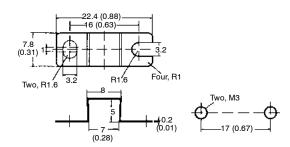
Material: Stainless steel (SUS304) Mounting Holes
