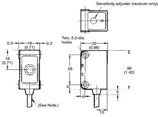
Note: Vinyl-insulated cable, 3.9 dia. Emitter has 2 conductors, Receiver has 3 conductors
