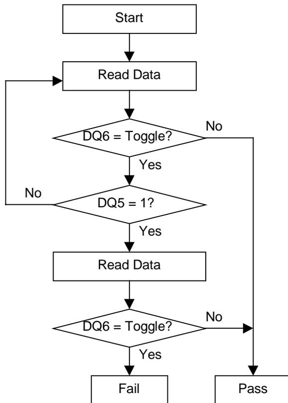
**Flowchart 7. Temporary Block Unprotect Algorithm**
