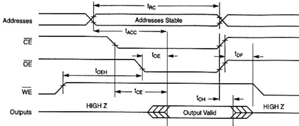
Figure 6. AC Waveforms for Chip/Block Erase Operations
