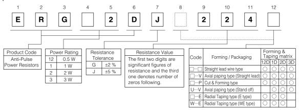
The above example shows an anti-pulse resistor, 2 W power rating, resistance value of 220 k ohms, tolerance ±5 %, and package of standard bulk packing.
