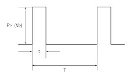
$\begin{array}{ll} P_P & : \text{Pulse limit power (W)} \\ V_P & : \text{Pulse limit voltage (V)} \\ \tau & : \text{Pulse continuous time (s)} \end{array}$
