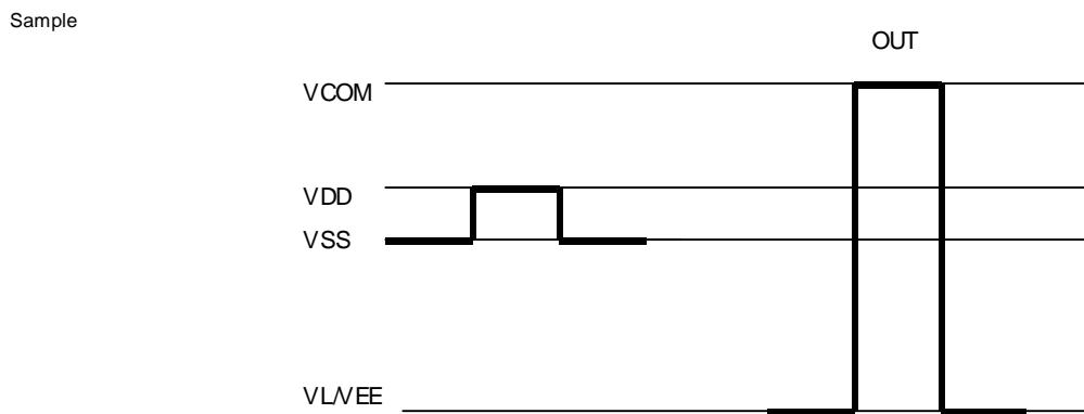
Logic input (CPV, OE, L / R, XAO, MODE, STV1, STV2) should be either at VDD or VSS.
